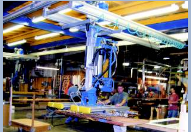
A ceiling mounted double girder system with vacuum lifter handles high end doors for the residential market.
